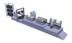
In pultrusion process the fibers are impregnated with a thermoset resin and pulled through a heated die where curing takes place
