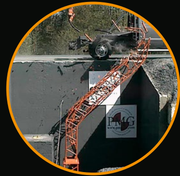
DYNAMIC IMPACT OF LATTICE MAST
